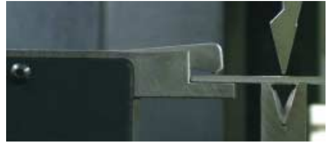
E-Bend S measuring cycle takes only 2.5 s.
